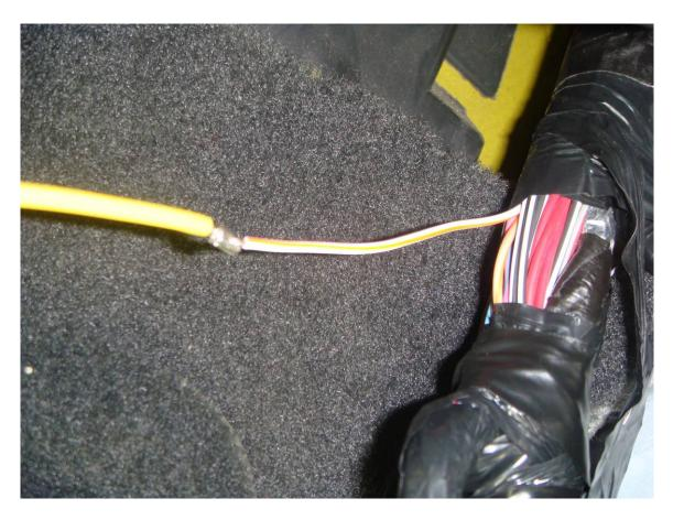
36. Carefully, route the two wires up the kick panel and across the bottom of the dash. Make sure to tape and zip tie the wires securely.
