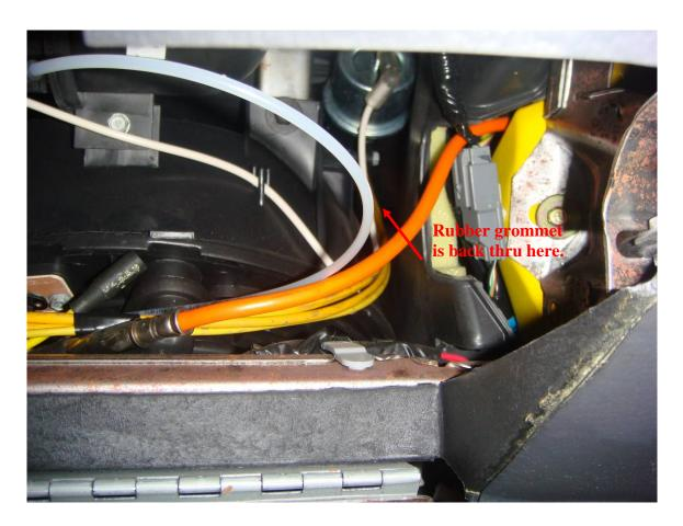
9. Feed the 3 wires through the opening in the inner fender to the engine compartment.
