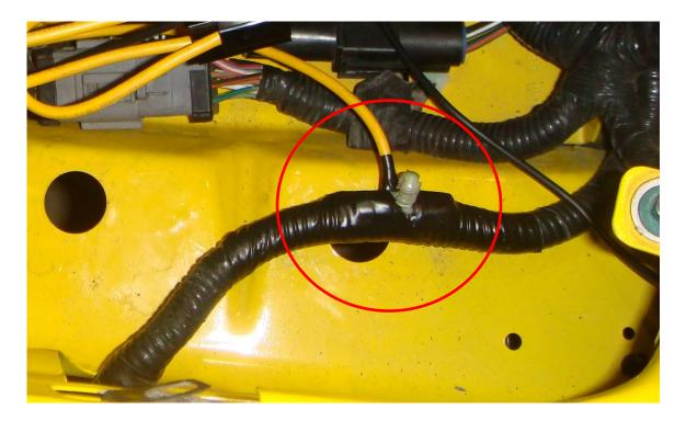
11. Unplug the black connector that is at the bottom of the fender area and locate Yellow wire with the Black stripe. Strip the insulation off of the wire and solder a new 12 ga. wire to the wire. This new wire should be cut to be about 18 inches long. When you are done, once again, tape the soldered connection, retape the loom, and reconnect the plug.
