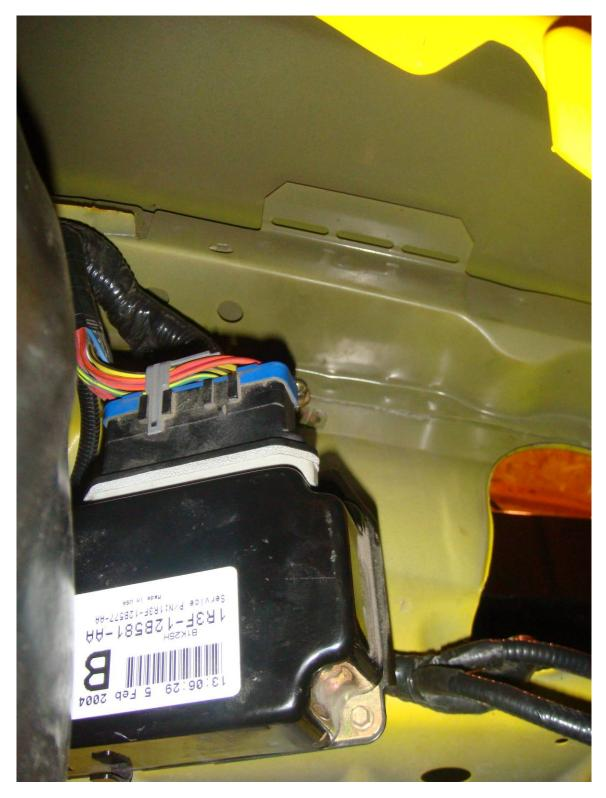
5. Remove the air filter and all intake parts in order to clean out the fender area. Also remove the auxiliary fuse box that is circled in the picture.
