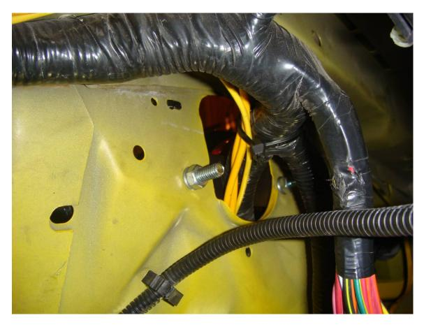
10. Remove the tape and wire loom and locate the **Orange** wire with **Light Blue** stripe. Remove the insulation from the wire and solder a 12 ga. strip of wire to it. This is another new wire and should be cut at least 18 inches long. When done, tape up the soldered connection and then the entire loom.
