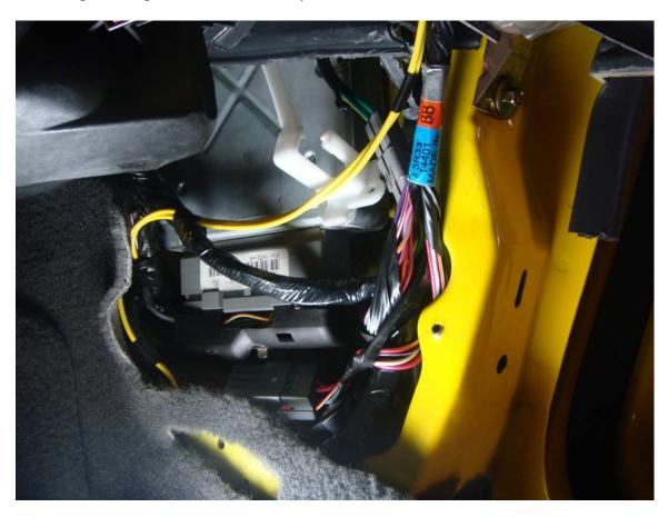
37. Route all of the wires under the dash and over to the center column. Make sure that are support and tucked away. There are now 5 wires in total -2 from the computer and 3 from the engine compartment.
