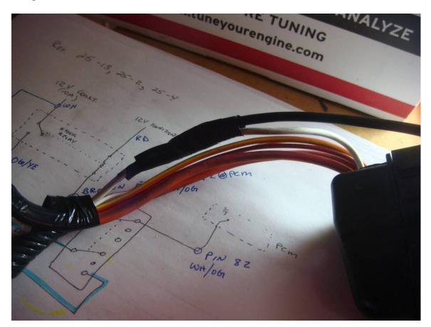
19. On the same harness, remove the insulation on the **Orange** wire with the **Yellow** stripe, solder a 12ga wire to it, and then tape the soldered connection and the entire wiring harness. The 12ga. wire should be about 12 inches long.
