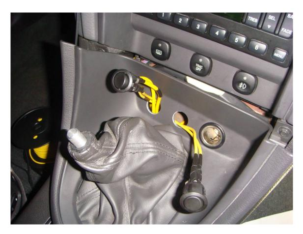
47. Reinstall the shifter bezel and press the switches into the holes. Make sure that their orientation is the way that you want them. (If you are consistent with top and bottom with my directions and install them that way, normal operation mode would be with both rocker switches in the up position – Fan off and IC pump in ECU control.)
