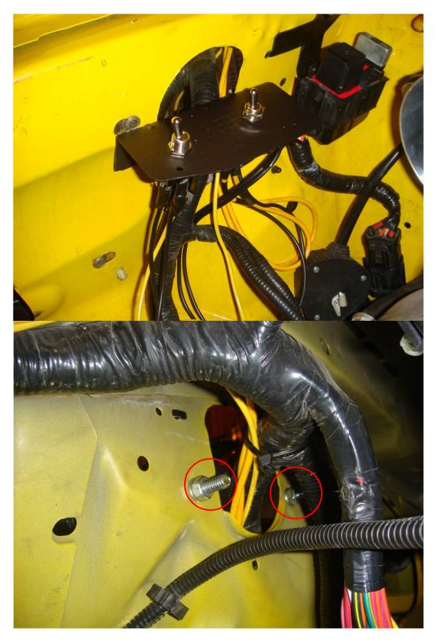
7. Cut 2 lengths of 12 ga. wire and 1 length of 16 ga. so that you have enough to run from the fender area to the shifter bezel with extra length to spare.
